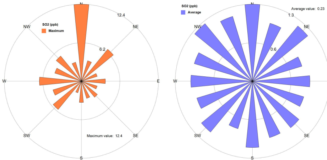
Figure 5.11 Maximum and Average SO 2 measurements by Wind Direction
