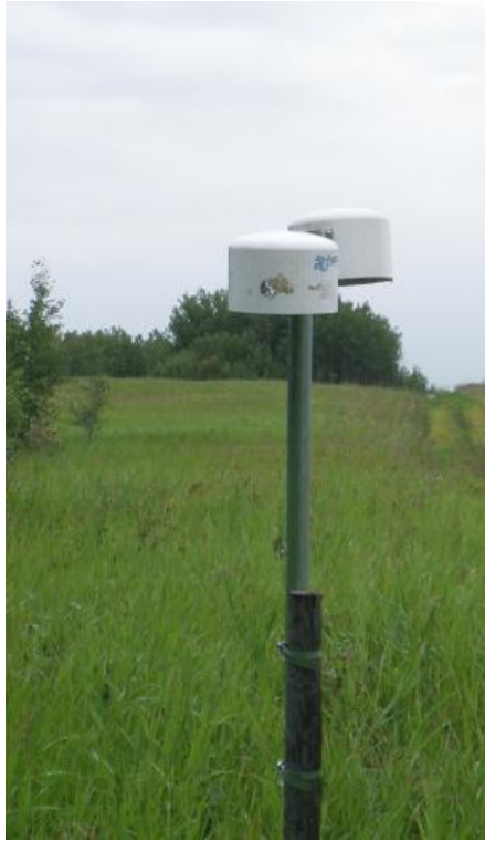
Figure 2. Duplicate Sampling Head Installed
